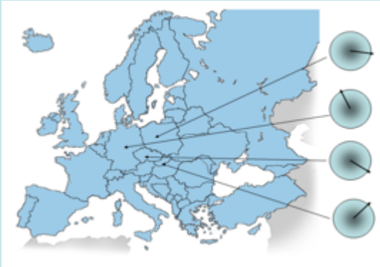
Wide Area Measurements (Field use of reference PMU)
