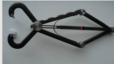
DLC coated surgical instrument
