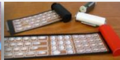
Rollable Canatu Nanocarbon sensor
