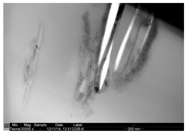
Diamonds retain their adhesion to h-BN during compounding and injection molding
