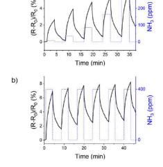
Figure 2 (a) relative signal to various concentrations of NH<sub>3</sub>, (b) relative signal to a repeated concentration of 400 ppm NH<sub>3</sub>
